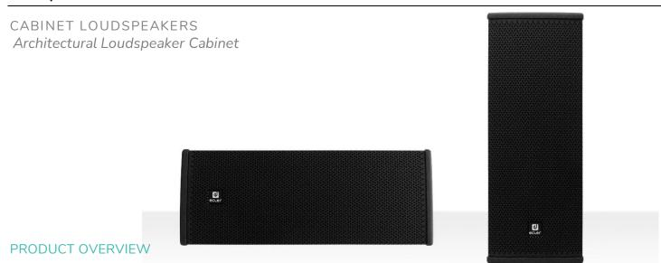
ARQIS205i is a 2-way wooden loudspeaker cabinet with a compact format, stylish aesthetics, excellent sound quality and long-term reliability, featuring 140 WRMS @  $8\Omega$ , 2 x 5" woofer and 1" HF Compression Driver. Its "U" shape wall bracket (included) allows for tilt adjustment. It has been specifically designed to fulfil permanent installation requirements where a perfect balance between sound performance and architectural/interior's design matching is a must.
