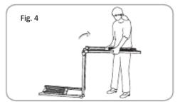
2. Unfold the frame until the latch on the hinge "clicks" into place. Repeat the procedure for the shorter sections.
