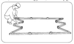
11. Again, press in the silver locking buttons. Then, pick up one end of the folding frame, and walk it to the other end, folding the longer sections into thirds.
